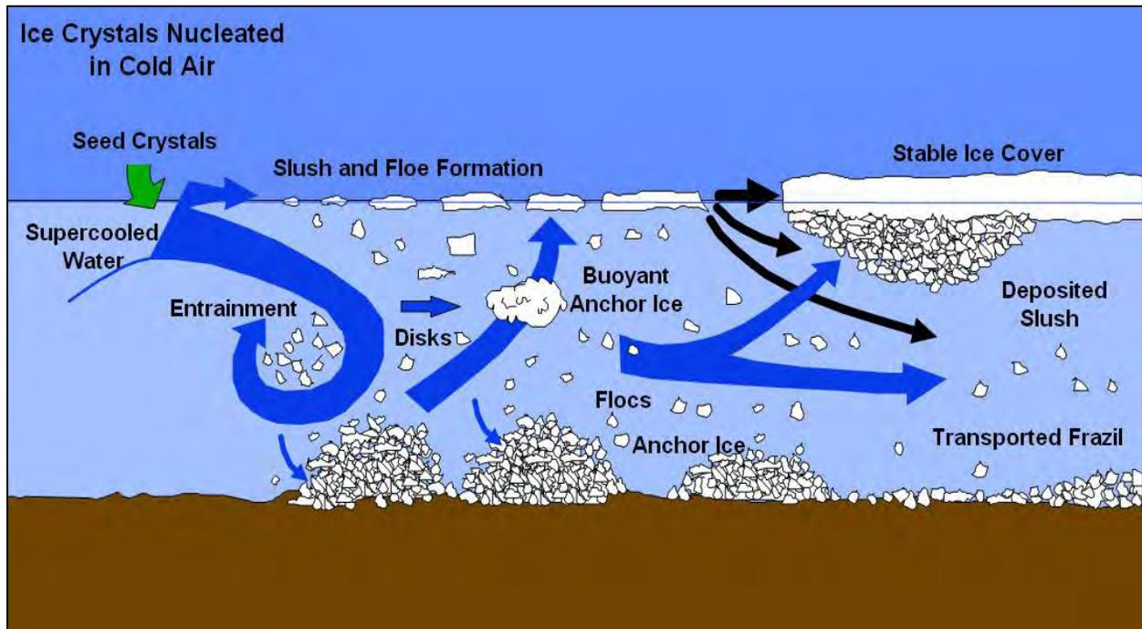
Figure 1. Forms of dynamic ice in flowing water include frazil disks and flocs, attached and released anchor ice, floating slush ice floes, and stable ice cover formation. Ice transported from upstream (frazil, released anchor ice, and flocs) may accumulate on the underside of a stable ice cover as an ice jam or hanging ice dam (shown here as “deposited slush”. Other types of dynamic ice not shown in this figure include ice weirs, ice dams, and aufeis<sup>1</sup>. From Daly (2002).
