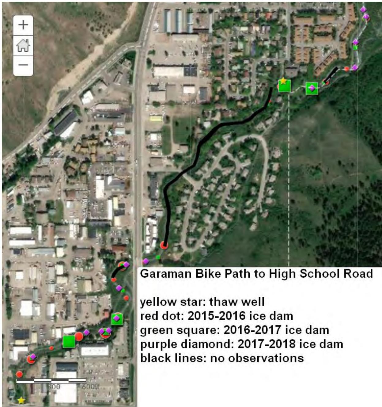
Figure 10. Anchor ice dams mapped between the Garaman Bike Path and High School Road between November 2015 and February 2018. This figure was generated from Alder Engineering's ArcGIS website (2018). The variation in marker size for the 2015-2016 and 2016-2017 data represent the relative number of observations of each individual anchor ice dam.
