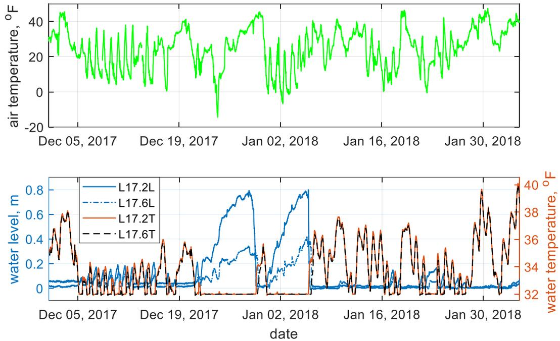
Figure 7. Top: winter 2018 Jackson air temperatures. Bottom: water levels (blue) and water temperatures at level logger stations L17.2 and L17.6 during the 2017/2018 winter.
