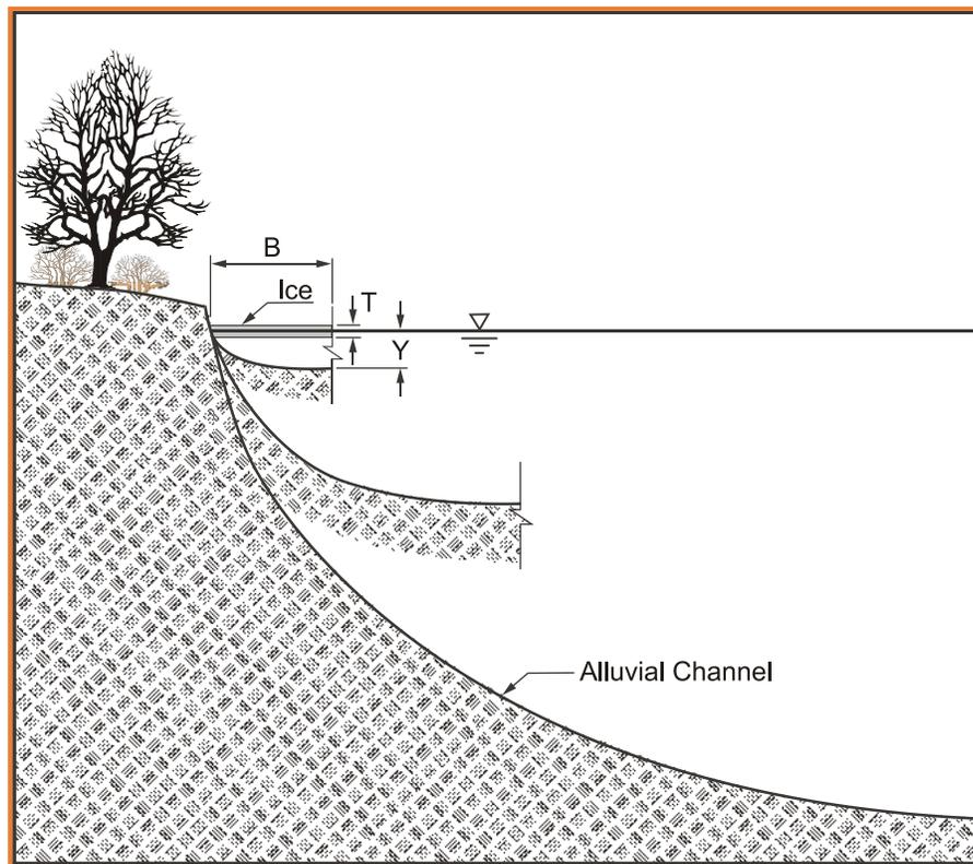
Figure 2. Diagram illustrating the effect that ice of a given thickness,  $T$ , has on different sized alluvial channels.  $B$  is distance from the bank,  $Y$  is the water depth, and the inverted triangle represents the water surface. For a small, shallow stream like Flat Creek, all ice has a very large effect on the flow depth. This effect is amplified when ice of given thickness also lines the channel's banks and bed, as further illustrated below in Figures 3 and 4. From Ettema (2007).
