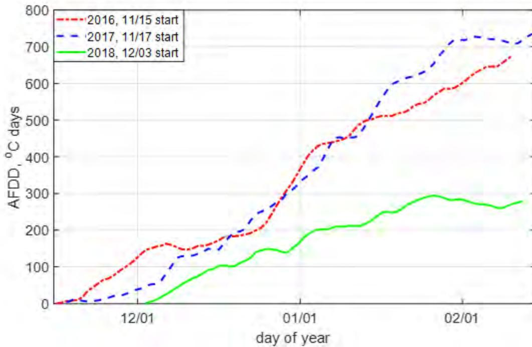
Figure 6. Plot of accumulated freezing degree days (AFDD) for winters of 2015-2018. The dates listed in the figure legend are the start time for AFDD. Winter totals are 11/15/2015 to 2/10/2016: 677 AFDD, 11/17/2016 to 2/16/2017: 750 AFDD, 12/3/2017 to 1/20/2018: 295 AFDD.
