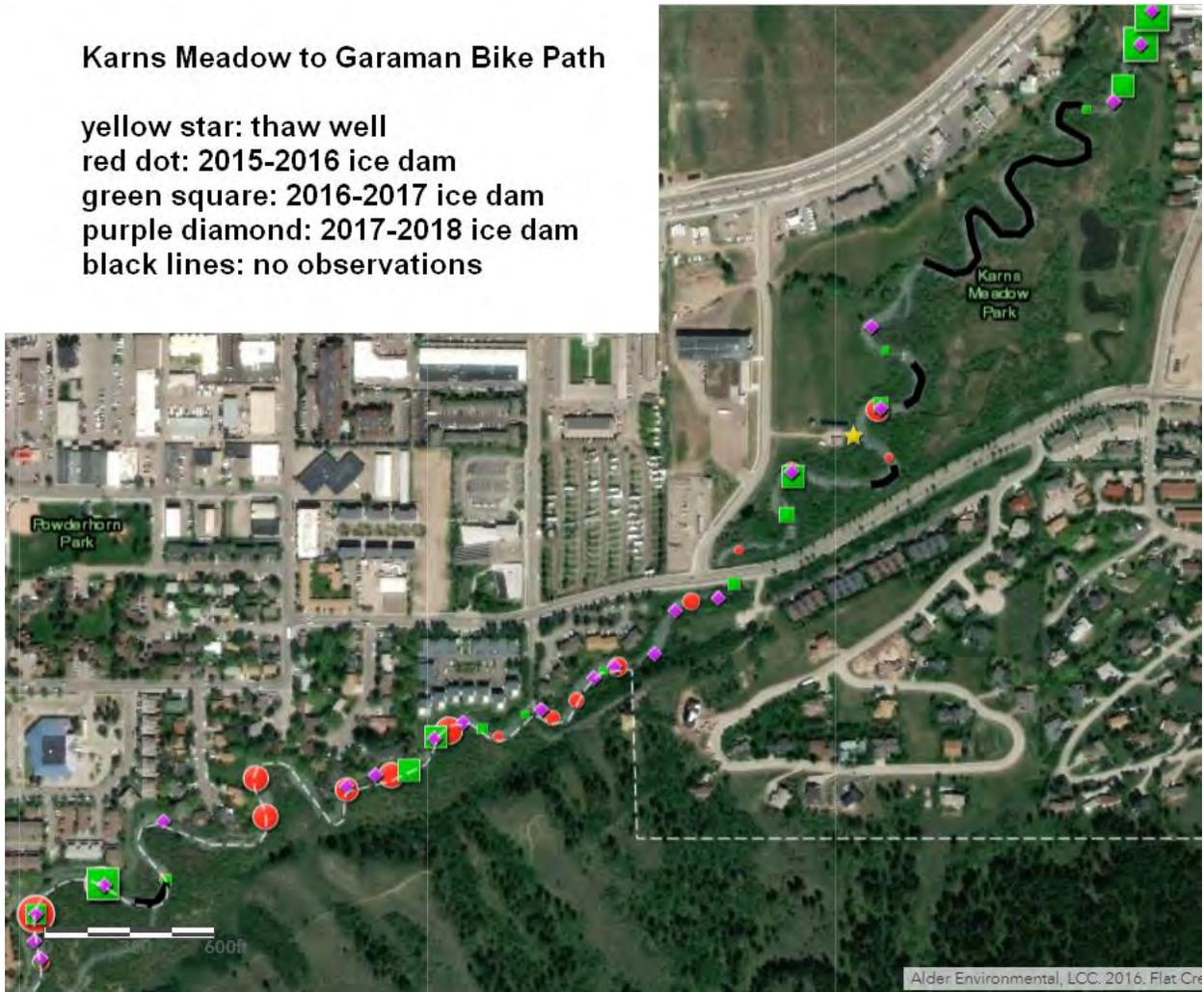
Figure 11. Anchor ice dams mapped between Karns Meadow and the Garaman Bike Path between November 2015 and February 2018. This figure was generated from Alder Engineering's ArcGIS website (2018). The variation in marker size for the 2015-2016 and 2016-2017 data represent the relative number of observations of each individual anchor ice dam.
